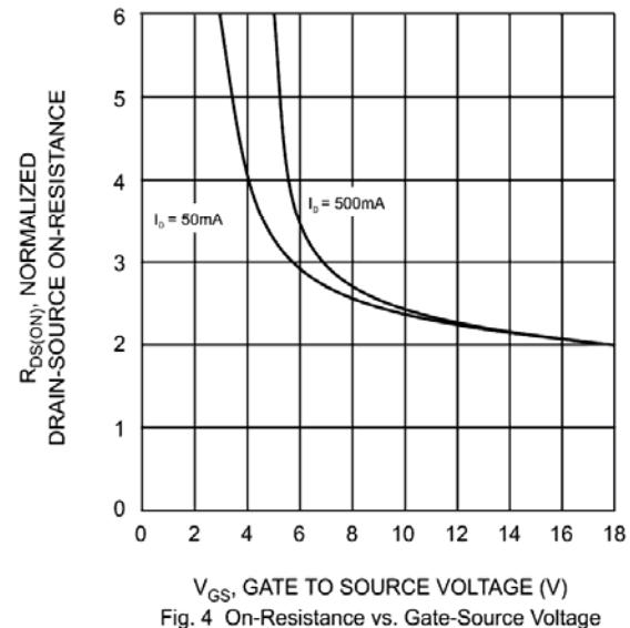
Fig. 4 On-Resistance vs. Gate-Source Voltage
