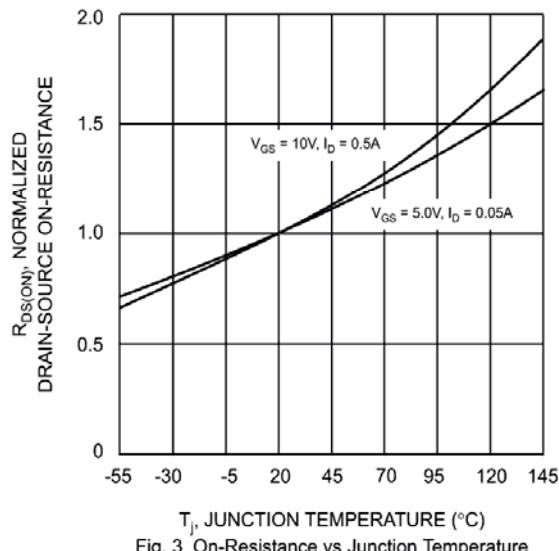
Fig. 3 On-Resistance vs Junction Temperature
