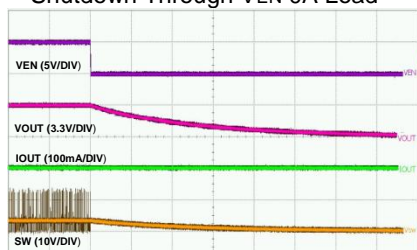
Shutdown Through VEN 0A Load
