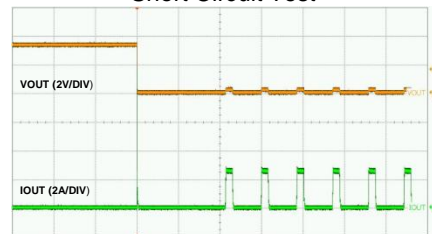
Short Circuit Test
