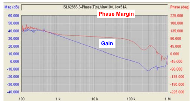
FIGURE 57. REFERENCE DESIGN LOOP GAIN T2(s) MEASUREMENT RESULT
