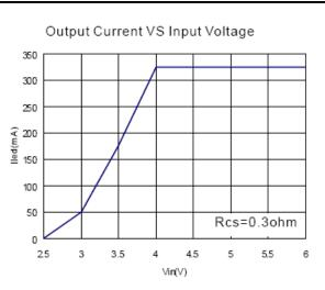
Output Current VS Input Voltage
