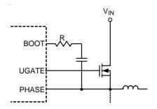
Figure 3. Reducing the UGATE Rise Time
