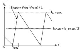
Figure 1. Boundary Condition of CCM/DCM
