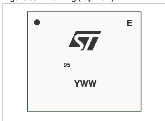
Figure 53. Marking (top view)
