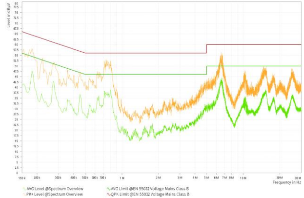
Figure 50: Neutral (Based on EN55032 Class B) V_{IN} = 230V_{AC} , V_{OUT} = 58.8V , I_{OUT} = 9.5A , f_{sw\_LLC} = 100kHz , average = green, QPK = red
